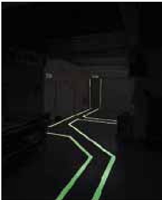
Figure 56: A way-guidance system
